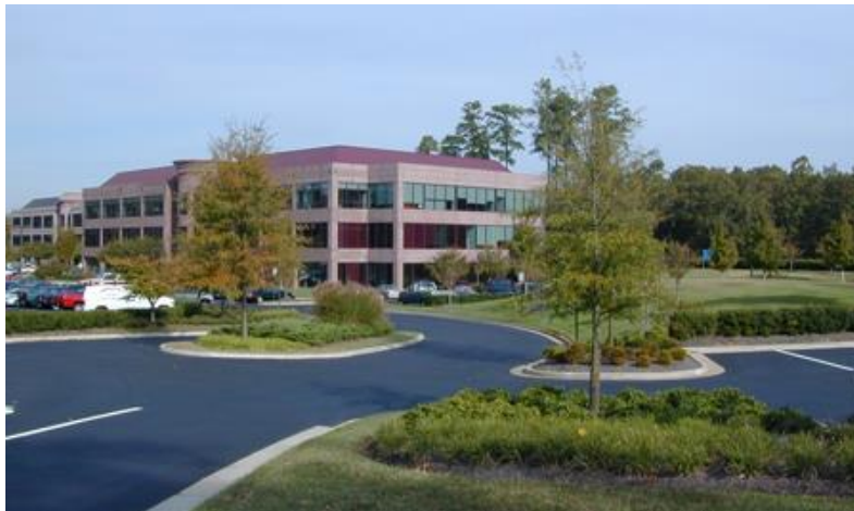
Figure 8.5-1: Landscaping and screening is intended to soften the appearance of large expanses of parking areas and can also provide areas for stormwater management.
