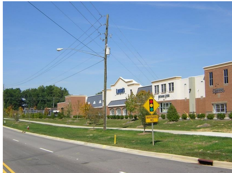
Figure 6.1-3: The buildings in the above images contain pilasters, cornices, and a series of façade setbacks (recesses) to visually break up the appearance of large facades.
